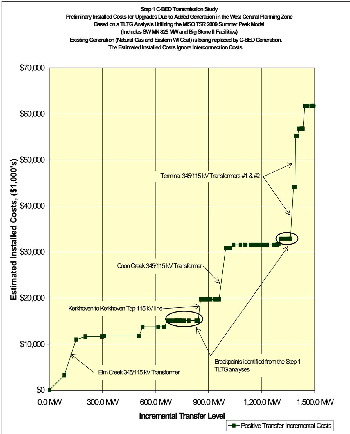
Figure 2: Step 1 TLTG analysis from 0 MW to 1,500 MW with Breakpoints for AC analysis Identified.
