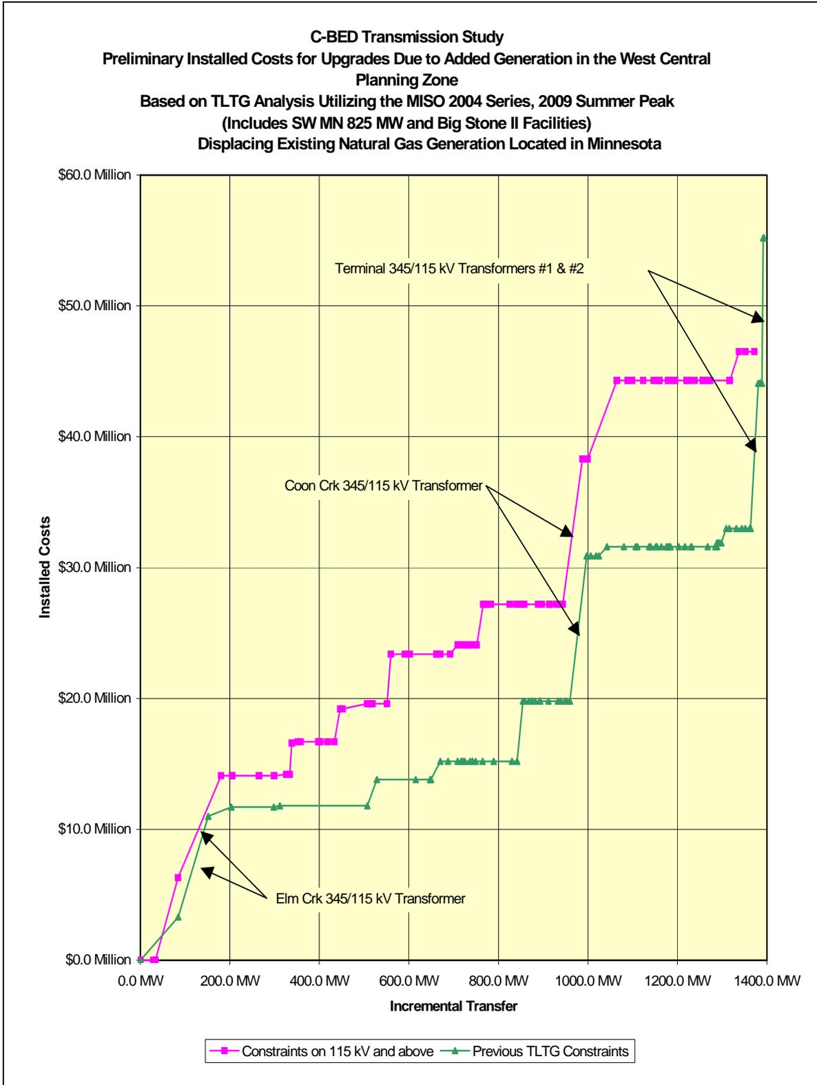
**Figure 3: Results of the Step 2 TLTG from 0 to 1,400 MW compared with the Step 1 TLTG Results.**
