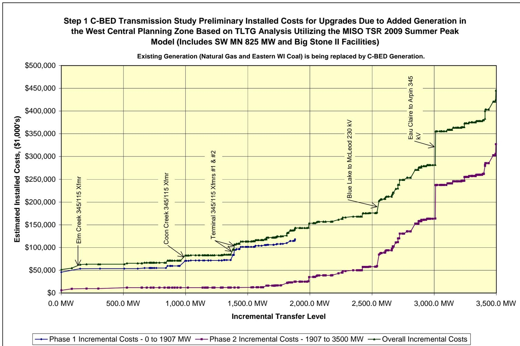
Figure 1: Results of the Step 1 TLTG Analysis from 0 MW to 1,907 MW and 1,907 MW to 3,500 MW.
